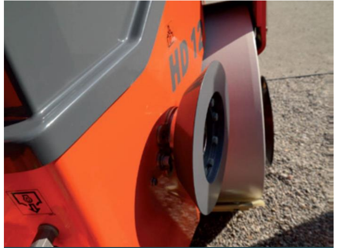
Figure 3 - Rouleau de compactage de joint (CRR, 2018)
