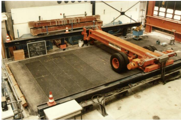
Fig. 1: View of the full-scale accelerated loading testing (ALT) facility
