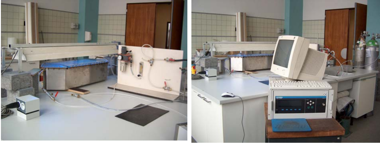
Fig. 1 Set-up of the test to determine the air purifying properties with large container (3*2 rows of pavement blocks)
